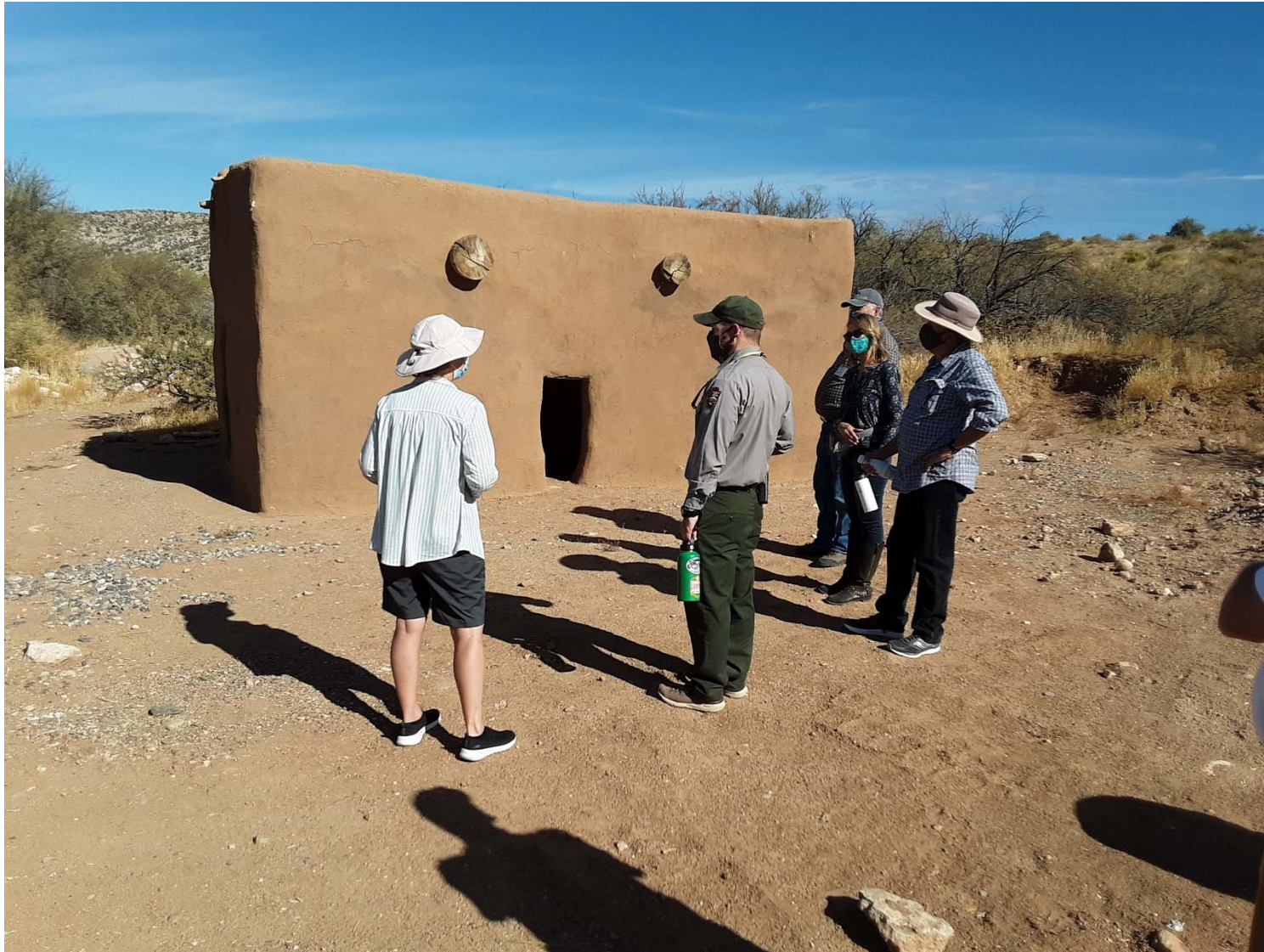
Experimental test room modeled after a room in Montezuma Castle, built to test building methods and materials. Used for fire test.
